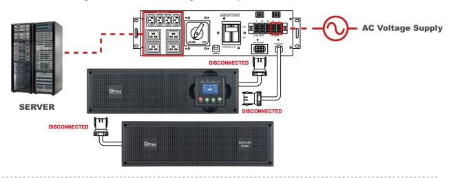
After Main UPS is uninstalled, Main UPS will be available to service center for repair. Individual PDU module will keep supplying AC power to loadings without interruption.
