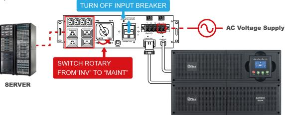
Disconnect the cable of Main UPS from PDU and battery bank.
